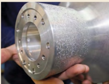
Drums are machined, drilled and needle-peened before dispatch for anodising
