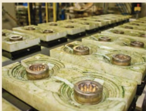
Raw gear punchings require machining down to the correct tolerances
